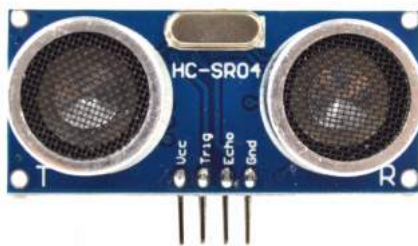
(a) Ultraschall-Modul HC-SR04
