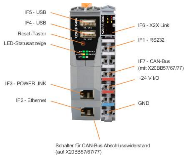
Abbildung IV.7: X20 Compact-S CPU (X20CP0484-1)
